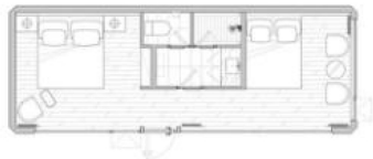
Model: B12 Length: 9.5m width: 3.3m height: 3.2m. Building area: 31.35m 2 .
