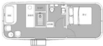
Model: A61 Length: 8.5m width: 3.3m height: 3.2m. Building area: 28m 2
