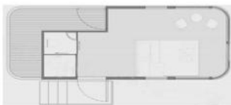
Model: B21 Length: 8m width: 3m height: 3m Building area: 24m 2
